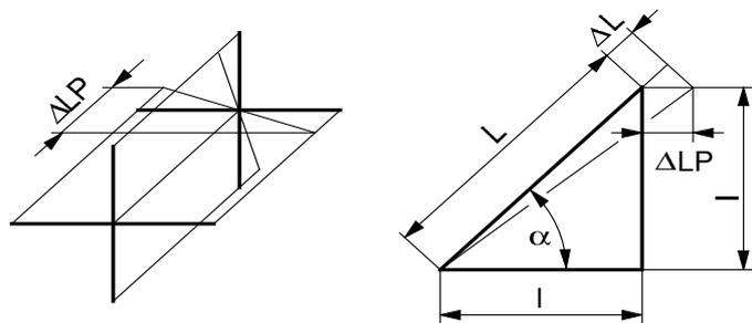
The error of straightness may be determined approximately with a length measurement in a diagonal direction at an angle of 45°. In the least favorable case the error of indication for size measurement is all alone caused by the error of straightness  $\Delta F_G$ . Because of  $L\cos\alpha=l/2$  and  $\cos^2\alpha=0,5$  for  $\alpha=45^\circ$  it is just as great as the error of indication for size measurement of the length  $l$  of the straight line:
