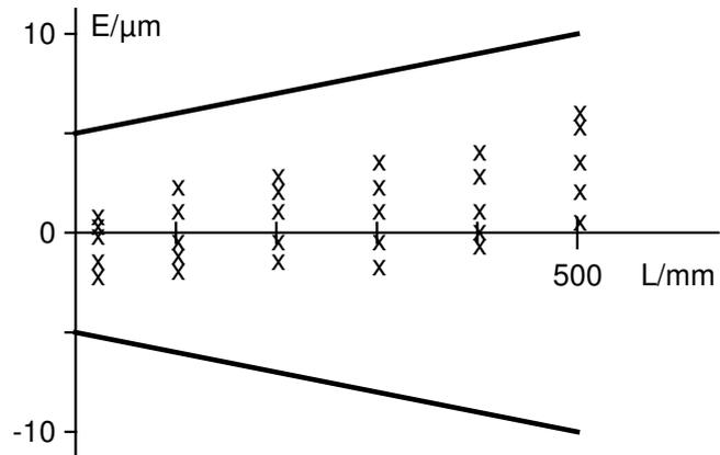
Measuring the distance between two parallel planes, the length dependent component  $L/K$  immediately represents the uncertainty contribution of the geometrical error of the CMM. Its maximum permissible error is derived dividing the nominal value of the length  $L$  by the factor  $K$ . The nominal value  $L$  is valid for all measurands that may be interpreted as a length or distance.
